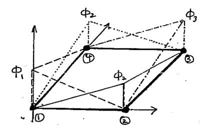
• Inter-element continuity at any point along any side has been assured due to the fact that the functional variation in the adjacent element has been defined in the same way and with the same coefficients.
