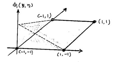
The variation along the element sides is linear. However within the element, the variation is not purely linear due to the cross term  $\xi\eta$
